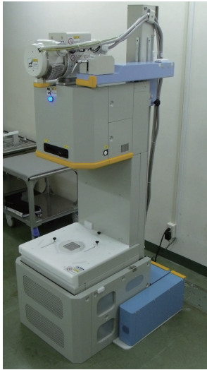
Fig. 3 Talbot-Lau interferometer for clinical evaluation of the imaging of limb joints.
